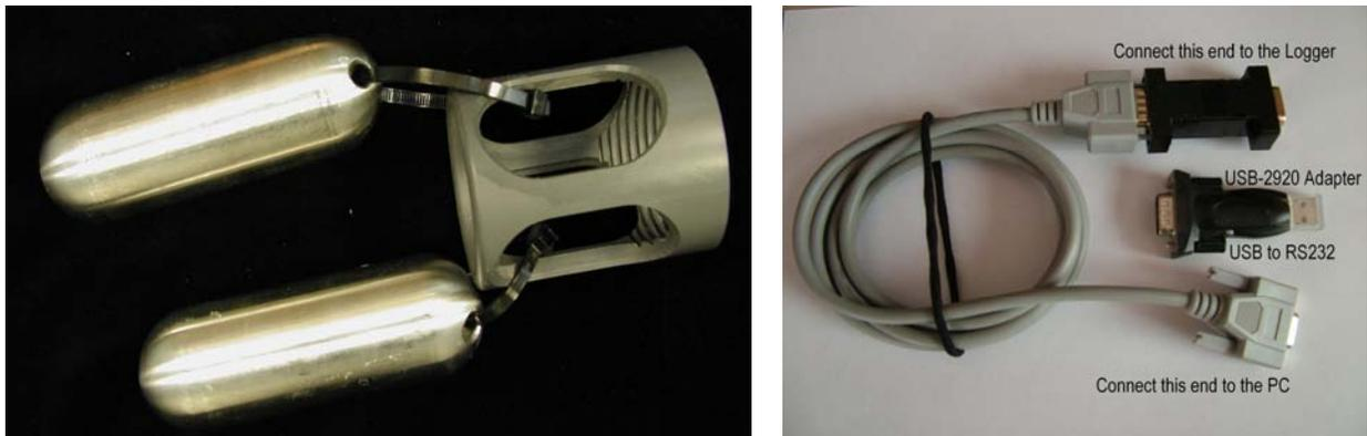
**Figure 7, Electrode shroud with attached weights, SIA Cable & Dongles**
