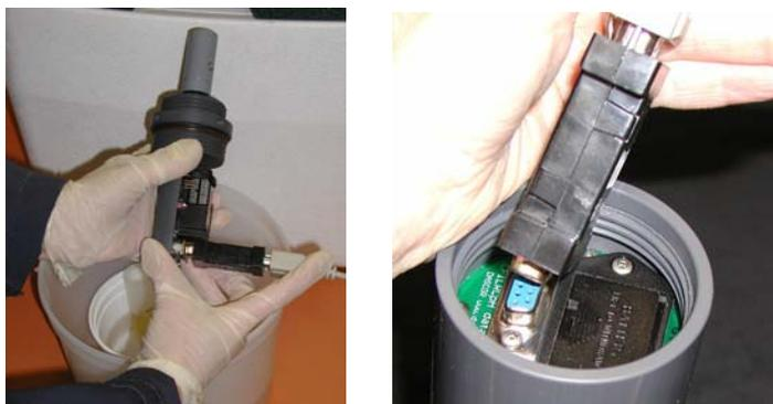
**Figure 35, Connecting the serial cable to the data logger (Type 3)**
