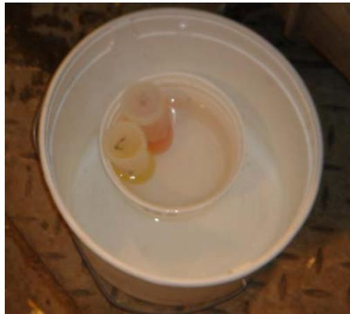
**Figure 10, Example of a warm water bath to keep cal-solutions at approximate rumen temperature**
