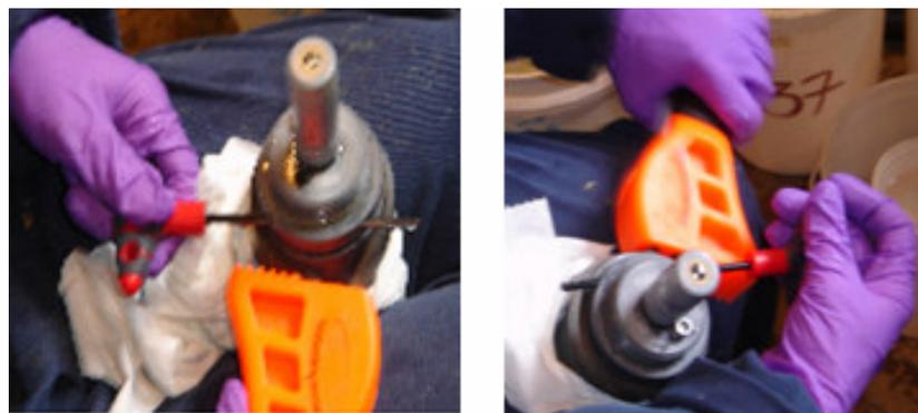
**Figure 34, Removing the cover from the original design LRCpH system**
