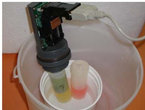
**Figure 15, Positioning of LRCpH system in calibration solutions**
