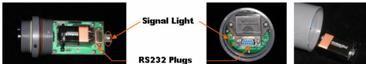
**Figure 3, Data logger (left: original model, right: new design)**
