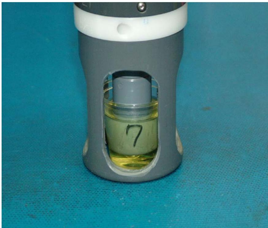
**Figure 46, Using the Shroud during Calibration**
