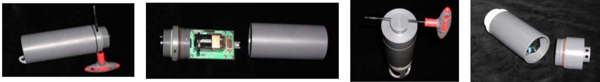
**Figure 4, Removing logger case (left: original model, right: new design)**
