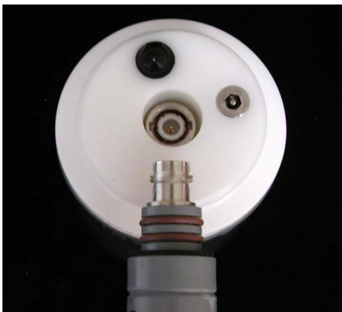
**Figure 9, Proper alignment for connection of pH sensors to the LRCpH system**
